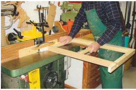
▲ Pic.24 The sashes need a groove in their outer top edges to clear the sash cords and pulley wheels
